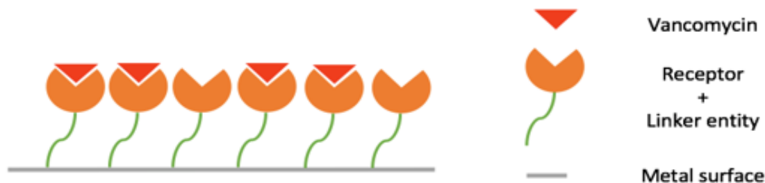
Figure 1: Schematics of metal sensor surface with immobilized receptors and vancomycin bound.
